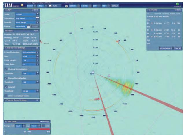
SUBEYE in anchor mode. Two suspicious objects are passively detected and their direction is shown on the display.
